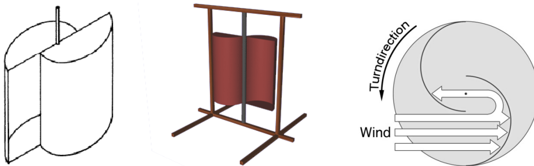
Fig. 2: Savonius rotor / wind power generator made out of oil barrels.
